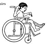
A simple wood or plywood chair can be easily made to fit the child's size and positioning needs. Repairs and replacements are easy because bicycle wheels and other standard parts are used (see p. 620).
