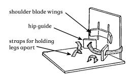
To seat the child, the frame can be put on the ground, a table, a chair, or into a wheelchair.
