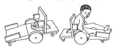
**Note:** The child's weight is over the large wheels. He can rock from one caster to the other. For travel over rough ground, he will learn to balance on the center wheel and barely touch down with the others.
