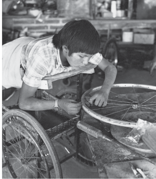
This boy with paraplegia from tuberculosis spokes a wheel for a wheelchair. He rides a wheeled lying board because of pressure sores on his butt.
