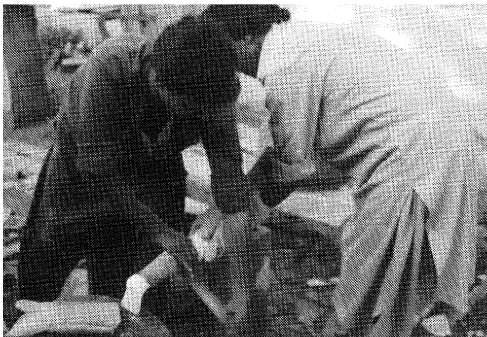
When the plastic is hot and soft, workers drape it over the plaster leg mold. Then they wrap it tightly with strips of rubber inner tube until it hardens (see p. 552).
