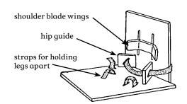
To seat the child, the frame can be put on the ground, a table, a chair, or into a wheelchair.
