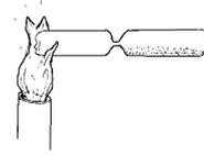
An easier method is to use a “soft glass” test tube, or a blood collection tube. Make a thin neck in the middle of the tube using a hot flame. You do not need to melt the open end — simply seal it with a cork or rubber stopper. This timer may be less accurate in a moist climate.
