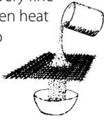
5. Put just enough sand in the tube so that it takes exactly 1 minute for all of it to run from one part to the other. Use someone's watch with a second hand to check this.
