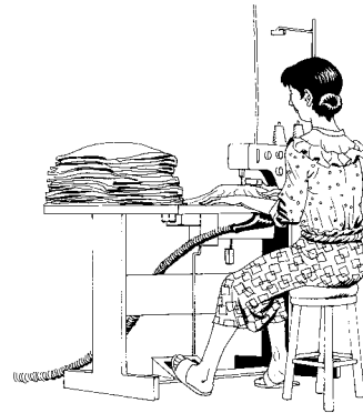
A local extractor removes the dust as it is created.
