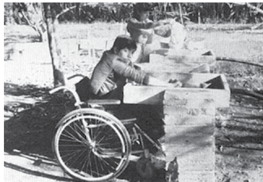
Outdoor washing area at PROJIMO—designed for work from a wheelchair.
