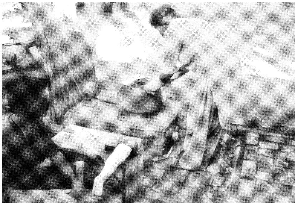
In Peshawar, Pakistan, the Community Rehabilitation Development Program makes leg braces from plastic bus windows. Here a worker heats the plastic over an outdoor mud stove.
