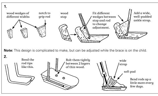
An adjustable wood brace for knee and ankle contractures
