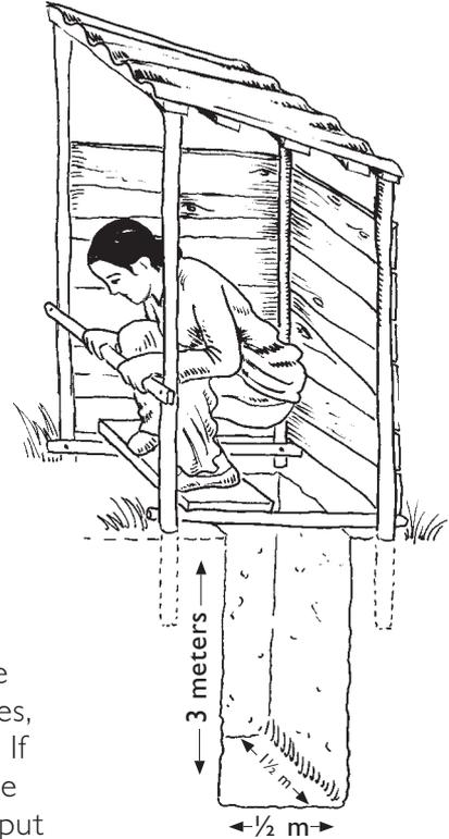
To be safe, a latrine should be at least 20 meters from all houses, wells, springs, rivers, or streams. If it must be anywhere near a place people go for water, be sure to put the latrine downstream.
