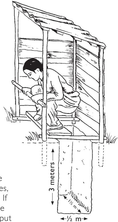
To be safe, a latrine should be at least 20 meters from all houses, wells, springs, rivers, or streams. If it must be anywhere near a place people go for water, be sure to put the latrine downstream.
